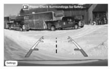
When the rear camera delay function is ON, it extends the display of the camera image into Drive mode until vehicle speed is greater than 5 mph (8 km/h). This is useful when trying to engage/disengage a trailer.
